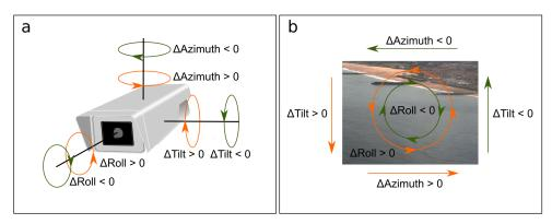
**Figure 5.** (a) Camera angle movements according to (b) azimuth, tilt, and roll deviations with respect to a reference image.
