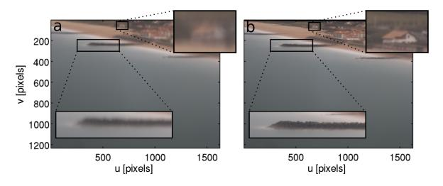
**Figure 8.** Time series average (spanning 1 October 2013–9 September 2018) of all of the (**a**) unstabilized frames and (**b**) stabilized frames of camera 2.
