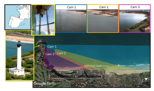
**Figure 1.** Map of Anglet Beach (Basque Coast, southwestern France) showing the location and field of view of the three-camera video system installed inside the Biarritz lighthouse (photo by M. Bourbon).
