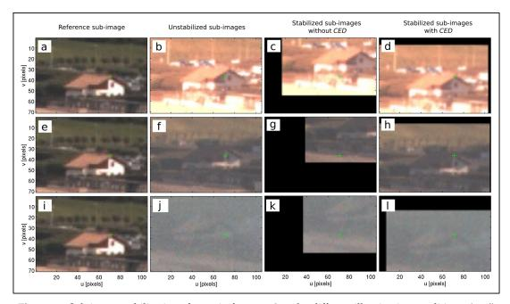
**Figure 10.** Sub-image stabilization of zone 1 of camera 2 under different illumination conditions. (**a,e,i**) Reference sub-image: 1 October, 2013—09:40:00 GMT; (**b,f,j**) unstabilized sub-images under shiny, cloudy, and foggy weather conditions; cross-correlation between the reference sub-image and the unstabilized sub-images with (**d,h,l**) and without (**c,g,k**) using the *CED*. The green cross represents the static keypoint that should match between frames.
