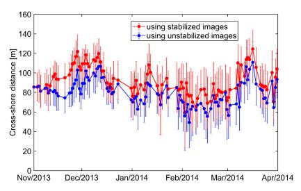
**Figure 11.** Daily alongshore averaged shoreline position extracted from stabilized (red dots) and unstabilized (blue dots) geo-rectified images for the outstanding winter period of 2013/2014. The alongshore standard deviation of the cross-shore position is indicated by the vertical error bars.
