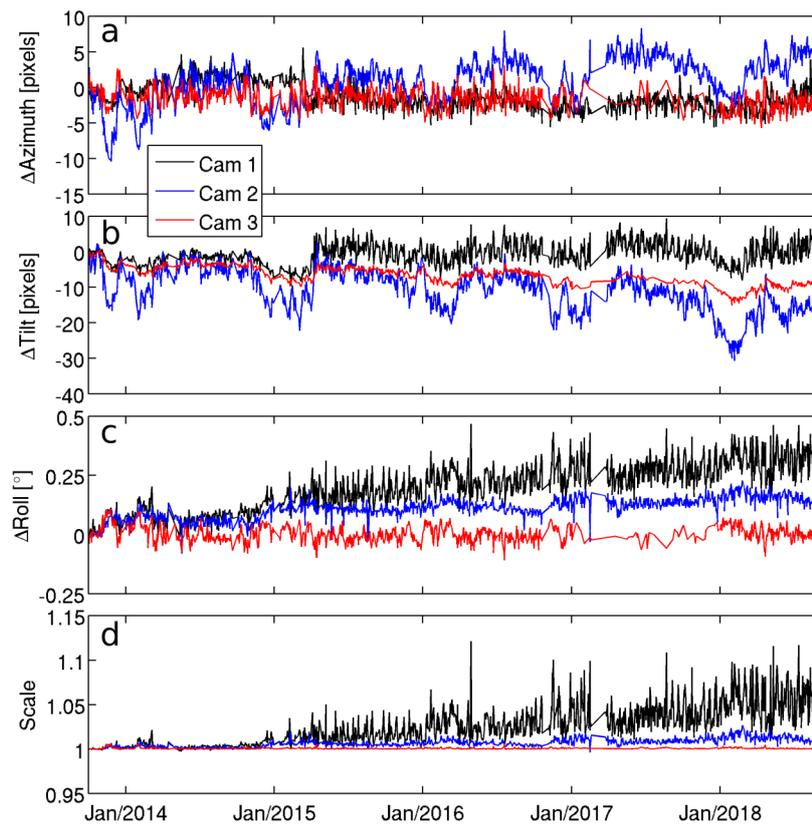
**Figure 7.** (a) Azimuth, (b) tilt, (c) roll, and (d) scale parameters of the similarity transformation matrix computed for the three cameras relative to the reference image: 1 October, 2013—09:40:00 GMT.
