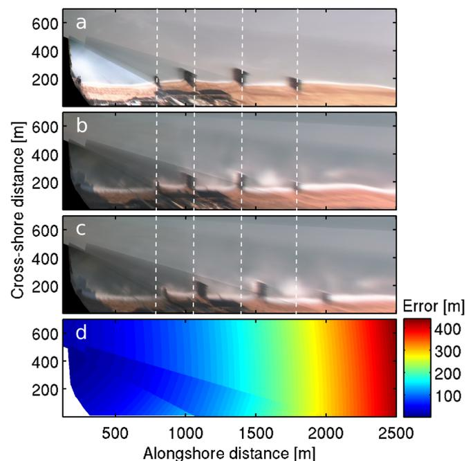
**Figure 9.** Anglet Beach geo-rectified time-exposure images highlighting the impact of camera viewing angle deviation. (a) Reference geo-rectified image: 1 October, 2013—09:40:00 GMT; (b) stabilized geo-rectified image: 6 February, 2018—09:15:00 GMT; (c) unstabilized geo-rectified image: 6 February, 2018—09:15:00 GMT; (d) positioning error due to camera movement for 6 February, 2018—09:15:00 GMT. White dashed lines indicate groins' original positions.
