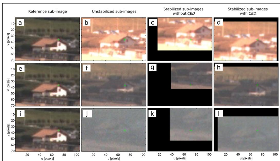
**Figure 10.** Sub-image stabilization of zone 1 of camera 2 under different illumination conditions. (a,e,i) Reference sub-image: 1 October, 2013—09:40:00 GMT; (b,f,j) unstabilized sub-images under shiny, cloudy, and foggy weather conditions; cross-correlation between the reference sub-image and the unstabilized sub-images with (d,h,l) and without (c,g,k) using the *CED*. The green cross represents the static keypoint that should match between frames.
