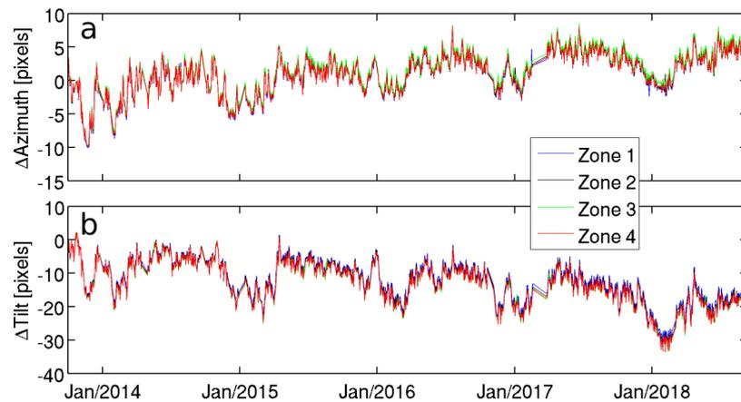
**Figure 6.** Daily (a) azimuth and (b) tilt displacements of the different sub-image zones in camera 2, expressed in terms of pixel shift. The deviations are computed with respect to the reference image: 1 October, 2013—09:40:00 GMT.
