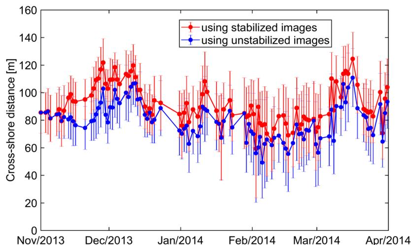
**Figure 11.** Daily alongshore averaged shoreline position extracted from stabilized (red dots) and unstabilized (blue dots) geo-rectified images for the outstanding winter period of 2013/2014. The alongshore standard deviation of the cross-shore position is indicated by the vertical error bars.
