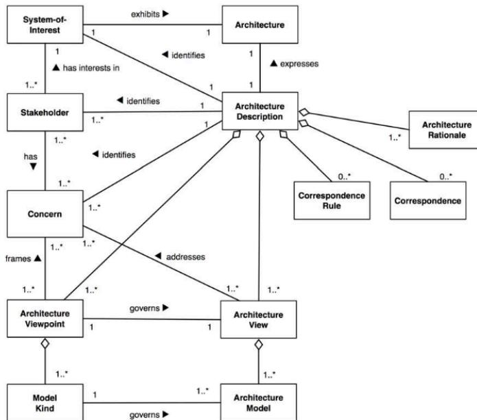
Fig. 3. Core ontology proposed by the standard ISO/IEC/IEEE 42010
