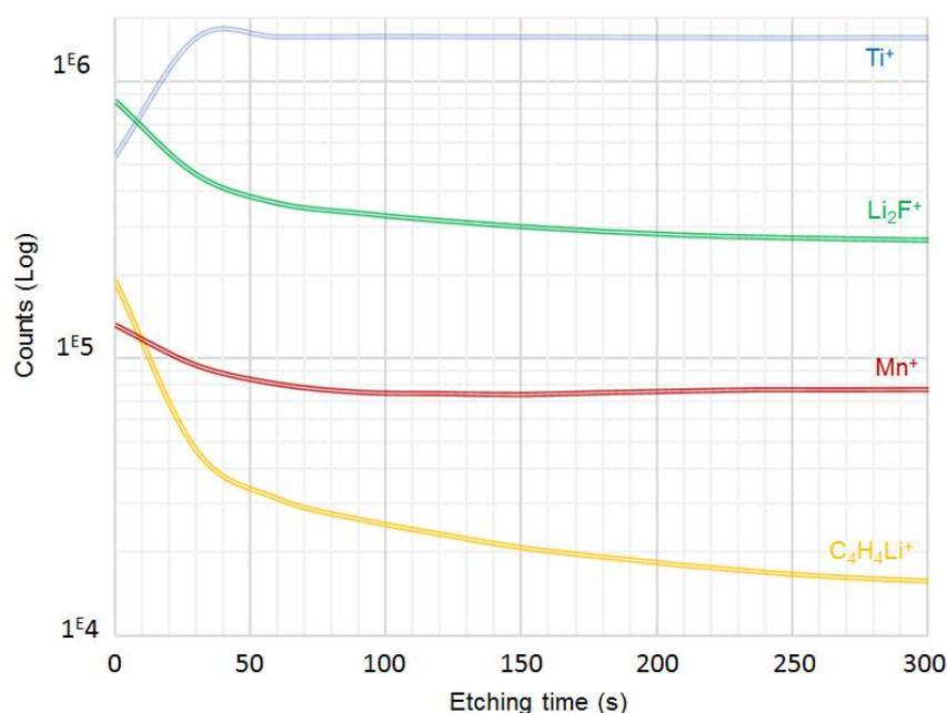
**Figure 4.** ToF-SIMS depth profiles of  $Ti^+$  (blue),  $Li_2F^+$  (green),  $Mn^+$  (red) and  $C_4H_4Li^+$  (yellow) secondary ions over 300 s etching time for the LTO/LMO system after the first cycle. (in color)
