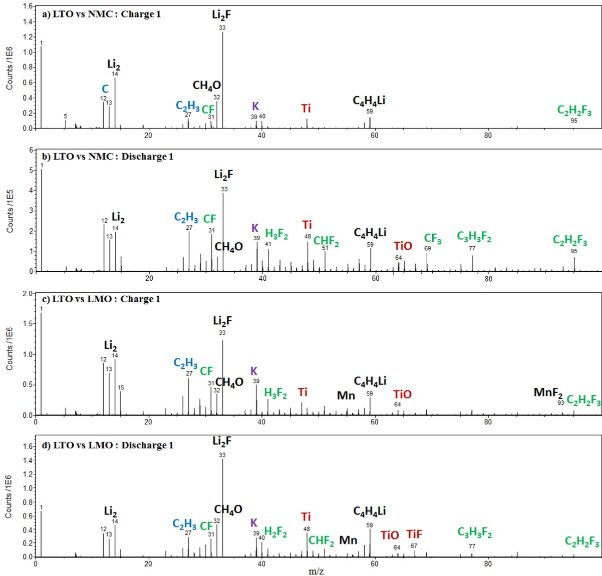
**Figure 2.** ToF-SIMS positive ion spectra over 0-100 m/z range for LTO electrodes cycled facing NMC after the first charge a), the first discharge b), and for LTO electrodes cycled facing LMO after the first charge c), and the first discharge d). (in color)
