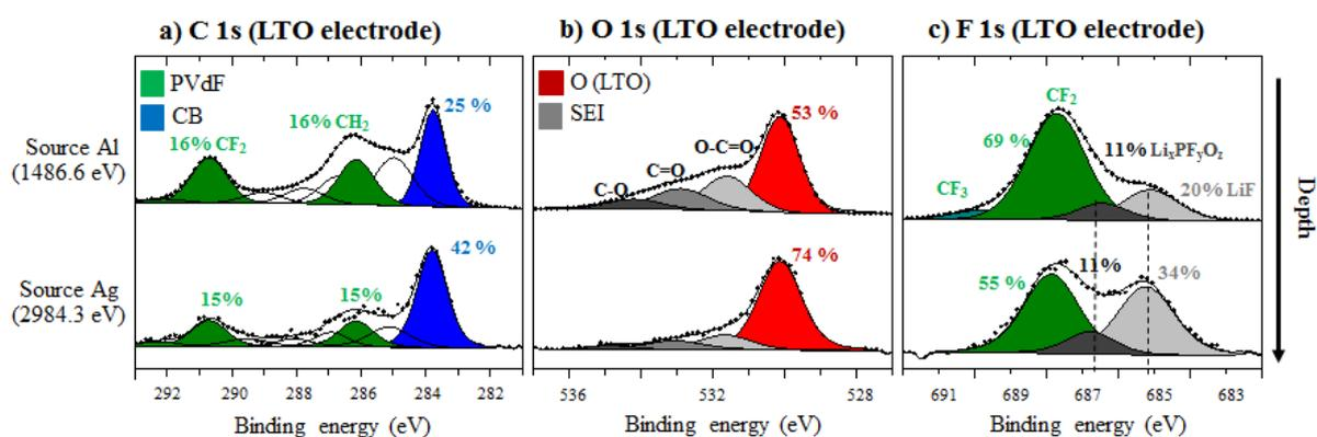
**Figure 6.** C 1s a), O 1s b) and F 1s c) XPS spectra of cycled LTO negative electrodes at the end of the first cycle in front of LMO electrode obtained with Al  $K\alpha$  radiation ( $h\nu=1486.6$  eV) (first line) and Ag  $L\alpha$  radiation ( $h\nu=2984.3$  eV) (second line). The relative percentages of main components are reported in the figure. (in color)
