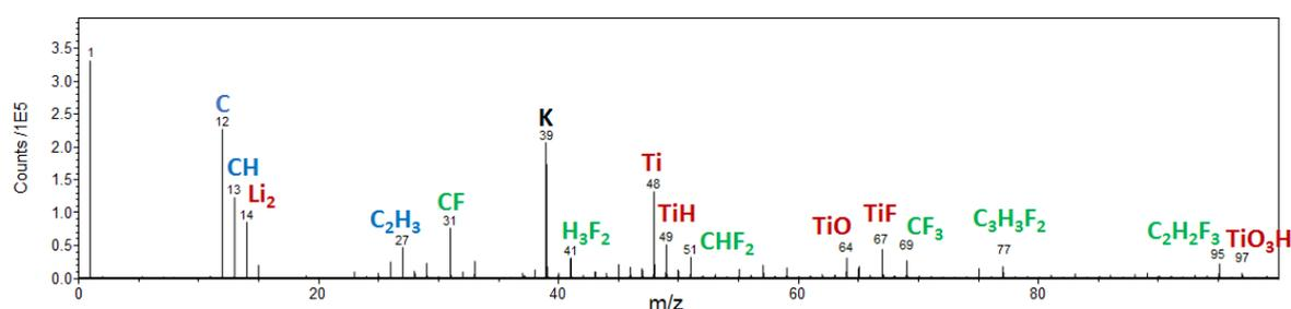
**Figure 1.** ToF-SIMS mass spectrum of the pristine LTO electrode over 0-100 m/z range in the positive polarity (blue, red and green peaks are attributed to carbon black, LTO active material and PVdF respectively). (in color)
