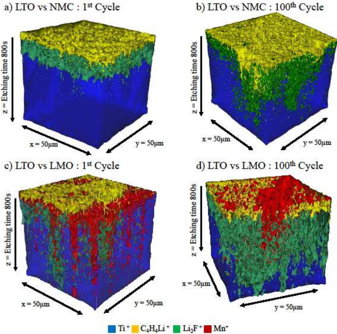
**Figure 5.** 3D images reconstruction from ToF-SIMS depth profile experiments showing the spatial distributions of Ti<sup>+</sup>, C<sub>4</sub>H<sub>4</sub>Li<sup>+</sup>, Li<sub>3</sub>F<sub>2</sub><sup>+</sup> and Mn<sup>+</sup> secondary ions over 50µm (x axis) by 50µm (y axis) raster size and 800s etching time (z axis), at the LTO electrodes surfaces at the end of the first and the hundredth cycles versus NMC electrode a) and b) and versus LMO electrode c) and d). (in color)
