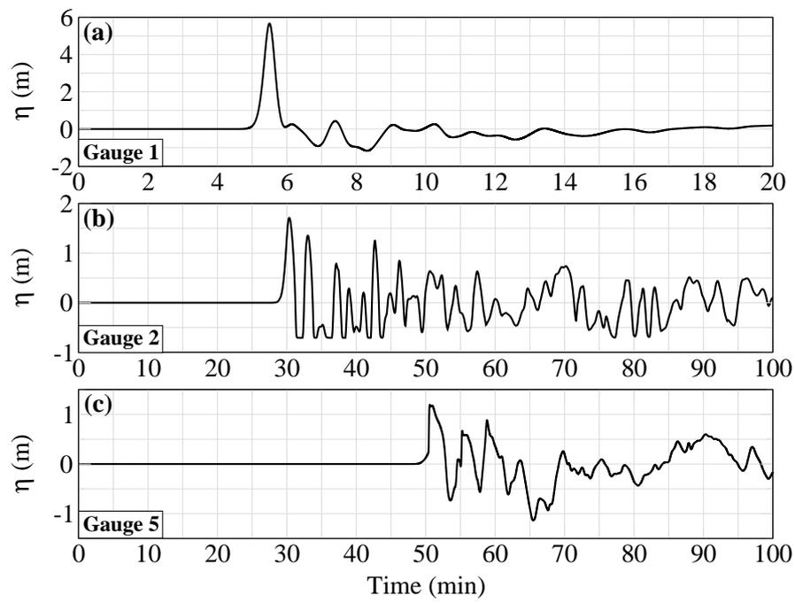
**Fig. 11** Computed surface elevations (m) **a** near the Anak Krakatau volcano, **b** at Tanjung Lesung and **c** at Kalianda (Gauges 1, 2 and 5, respectively, see Figure 9).
