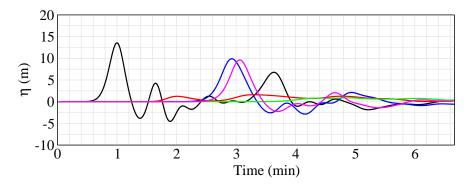
**Fig. 13** Time series of surface elevation calculated in the near-field by our model (150 million m<sup>3</sup> and the code AVALANCHE) at the Gauges 5' (black), 6' (blue), 7' (red), 8' (green) and 9' (magenta) used by Grilli et al. (2019) and presented in Figure 9b. Results are very similar to those presented in Figure 5e of Grilli et al. (2019).
