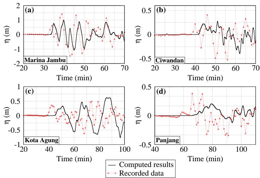
**Fig. 10** Comparison between recorded data (in red) and simulated water surface elevations (in black) at **a** Marina Jambu, **b** Ciwandan, **c** Kota Agung and **d** Panjang (Gauges 3, 4, 6 and 7, respectively, see Figure 9).
