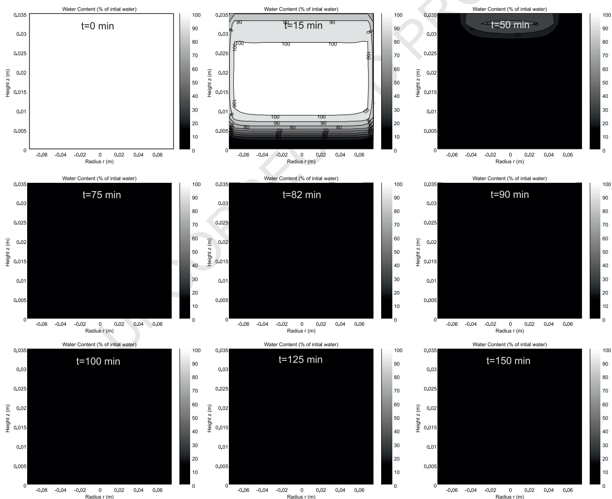
Figure 8. Evolution of the moisture content of the material within the basket as a function of space and time.
