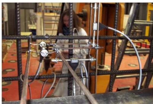
Location of the dual-coil vibrating-wire sensors
