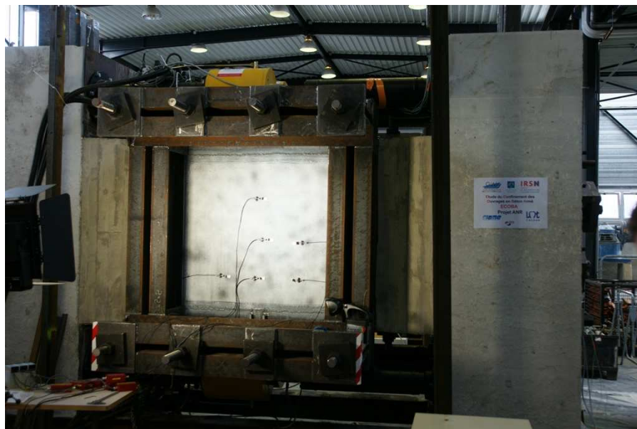
Figure 8 - DIC measurement system with the LVDT sensors
