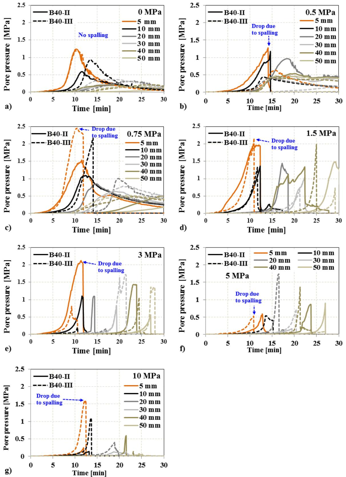
Figure 7 Development of pore pressure in B40-II and B40-III versus time at different depths.
