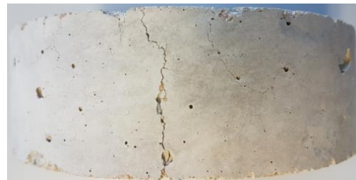
d) Image of B40-III preheated under a compressive stress \sigma = 5 MPa
