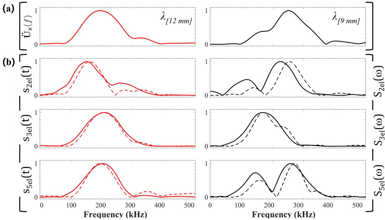
**Figure 9.** (a) Vertical acceleration recorded at 50 mm for two experiments performed with different apparent seismic velocities of  $2460 \text{ m s}^{-1}$  (left) and  $1850 \text{ m s}^{-1}$  (right). (b) Normalized seismoelectric observed (plain lines) and predicted (dashed lines) spectra for the different arrays and the two apparent velocities. The array length  $L$  was 10 mm.
