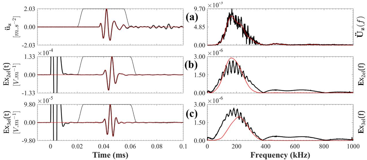
**Figure 4.** Vertical seismic accelerations (a) and seismoelectric data (b and c) displayed in the time domain before (black lines) and after tapering (red lines) with a trapezoidal time window and the corresponding spectra (right). The electric fields were deduced from voltage differences  $\Delta v_{2-el}(t)$  (b) and  $\Delta v_{3-el}(t)$  (c) after a division by the array length.
