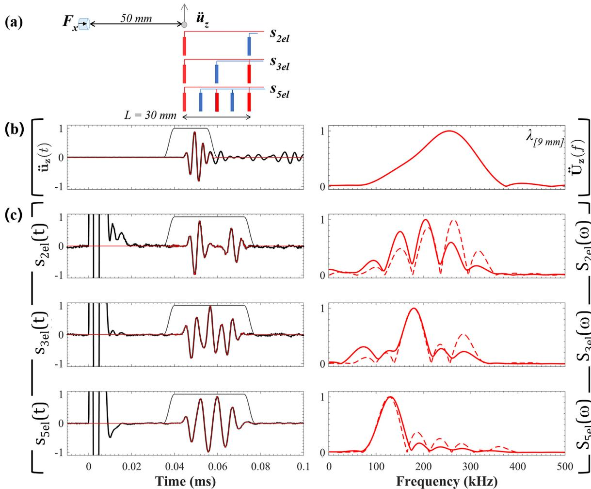
**Figure 8.** Influence of the number of electrodes involved in the recording array. (a) Sketch of the recording configuration. (b) Vertical acceleration recorded at 50 mm. (c) Seismoelectric measurements for the different arrays (left) and corresponding normalized observed (plain line) and predictions (dashed lines) spectra for two-electrode, three-electrode and five-electrode arrays, with an array length  $L = 30$  mm.
