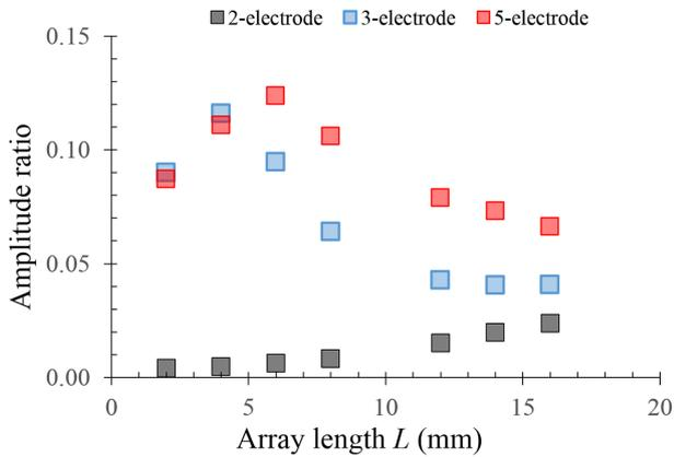
**Figure 16.** Amplitude ratio of interface response to coseismic electrical arrival according to array length for various array arrangements. The incoming seismic waves has a wavelength  $\lambda \simeq 9.1$  mm.
