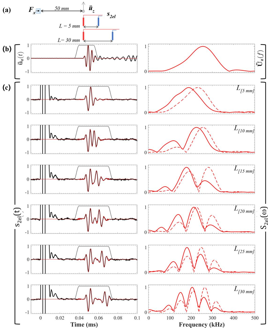
**Figure 6.** (a) Sketch of the acquisition for the two-electrode array. Outer electrode is displaced so that the  $L$  varies from 5 to 30 mm. (b) Seismic acceleration acquired at an offset of 50 mm (top) followed by (c) seismoelectric recordings for the different offset (left) and corresponding normalized observed (plain lines) and predicted (dashed lines) spectra (right).
