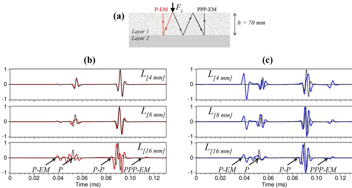
**Figure 15.** (a) Sketch of the two depth-generated seismoelectric disturbances. (b) Superimposition of the seismoelectric field (black) and the voltage difference (red) obtained for different array lengths. (c) Superimposition of the seismoelectric field (black) and the signal  $s_{3el}$  obtained for different array lengths. The inner electrode was located at an offset of  $-84$  mm. The  $P$ -wave wavelength equals approximately  $9.1$  mm.
