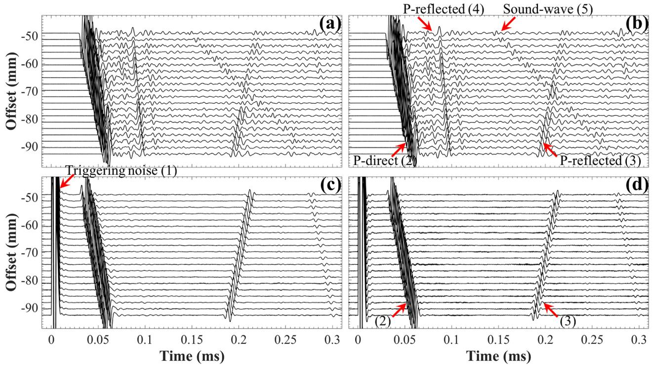
**Figure 3.** Seismic (a) and seismoelectric data (c) recorded with an array length  $L$  of 5 mm in the two-electrode configuration and generated with a source frequency of 200 kHz. (b) Seismic and (d) seismoelectric data recorded for the three-electrode configuration.
