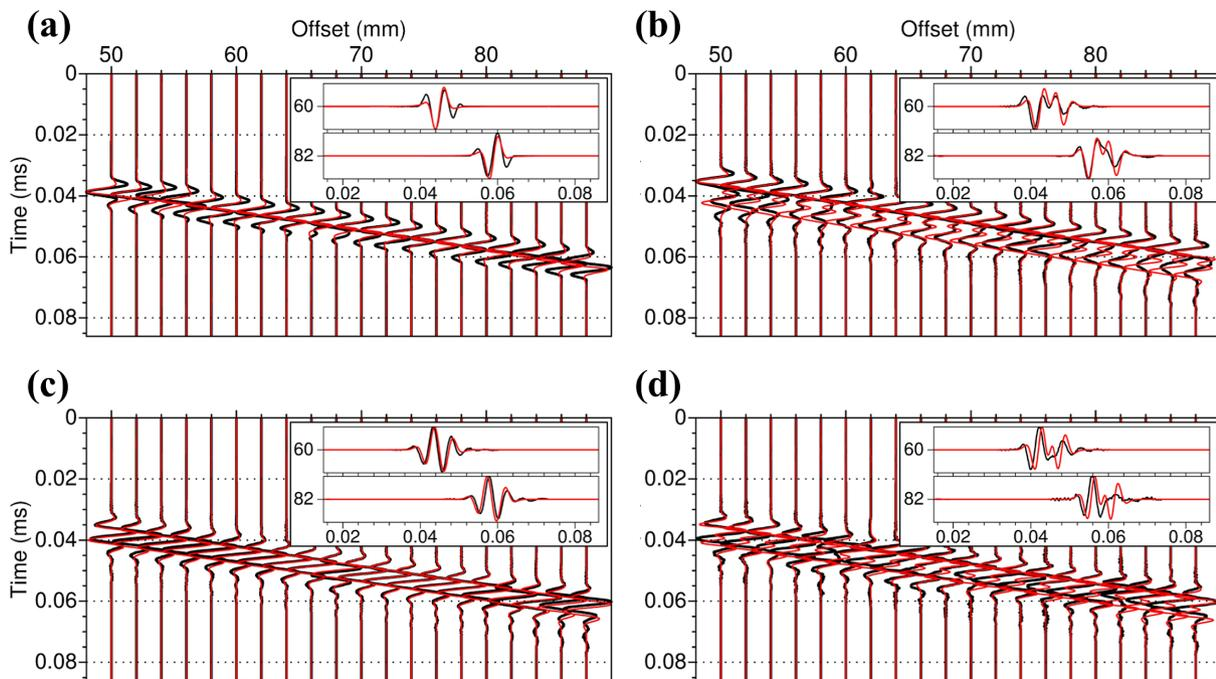
**Figure 11.** Comparisons between laboratory data (black) and numerical simulations (red) for the  $P$ -direct waves arrival propagating in material 1 with an angle  $\alpha \approx 40^\circ$ . (a) Vertical seismic acceleration. Seismoelectric data are displayed for two-electrode (b), three-electrode (c) and five-electrode (d) arrangements. The insets zoom in at two acquisition offsets : 60 and 82 mm.
