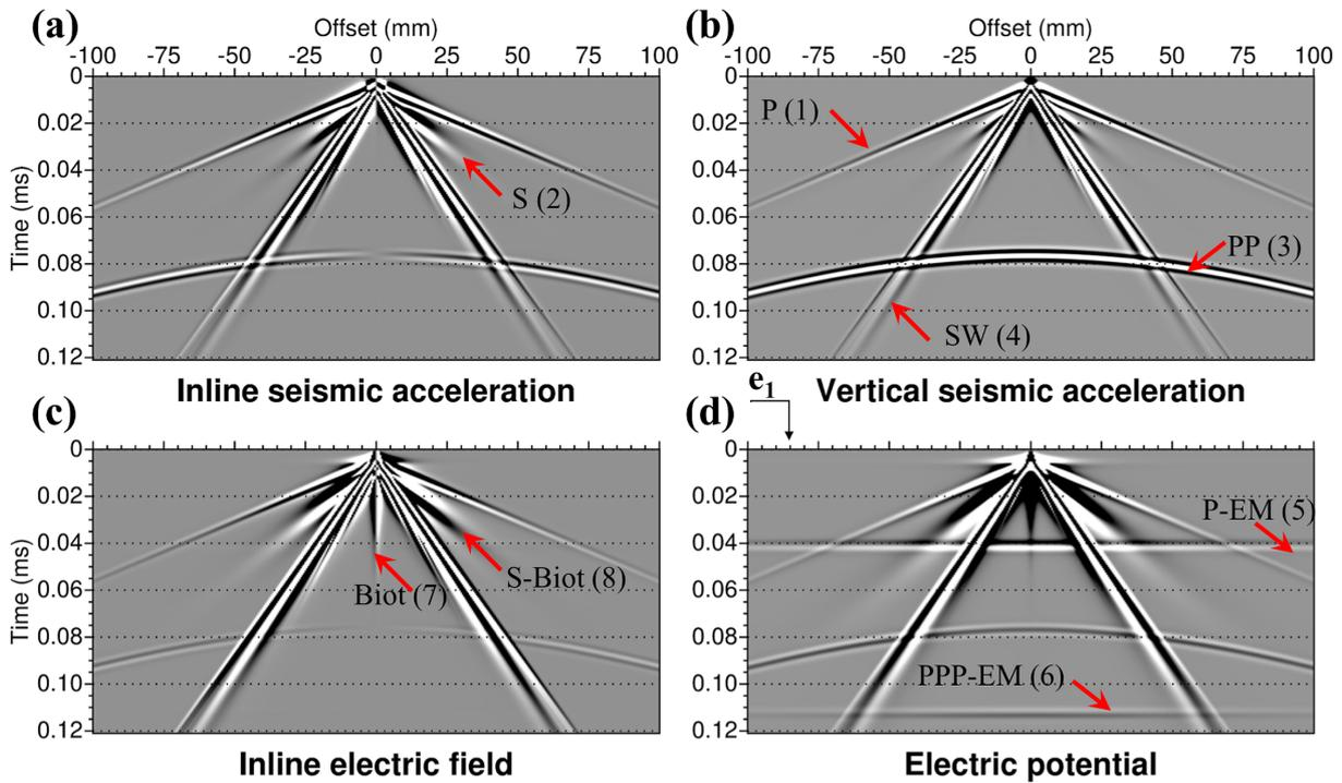
**Figure 14.** Numerical computations of longitudinal seismic acceleration  $\ddot{u}_x(t)$  (a), vertical seismic acceleration  $\ddot{u}_z(t)$  (b), seismoelectric field  $E_x(t)$ (c) and absolute electrical potential  $v(t)$  (d) generated by a vertical point source in a two-layer model.
