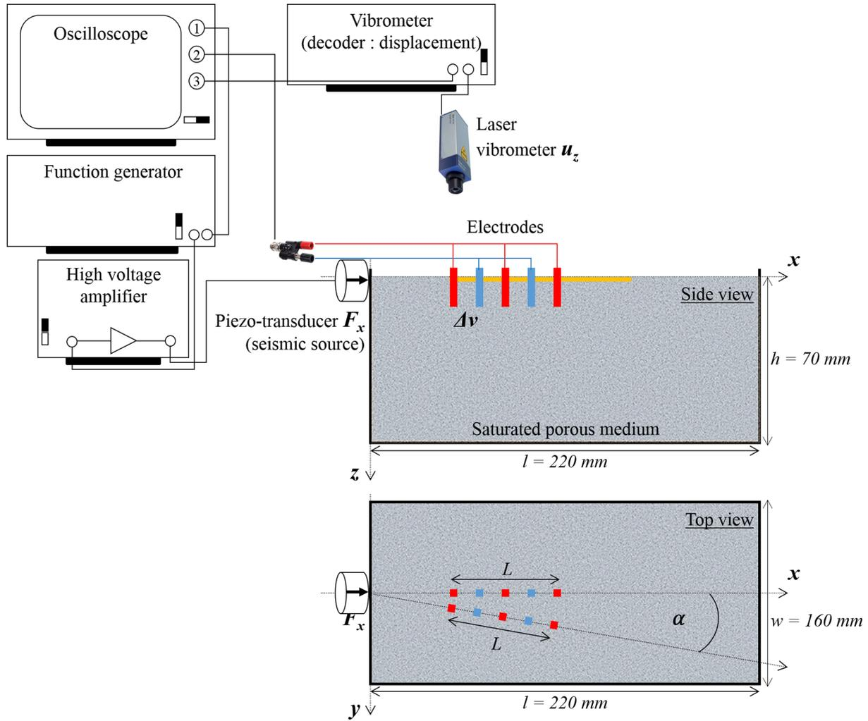
**Figure 1.** Side and top views of the laboratory experimental setup and the acquisition chain. A piezoelectric transducer generates seismic waves, whose surface displacements are recorded using a laser vibrometer while seismoelectric signals are recorded using electrode arrays. By rotating the receiver line by an angle  $\alpha$ , different apparent seismic velocities are generated.
