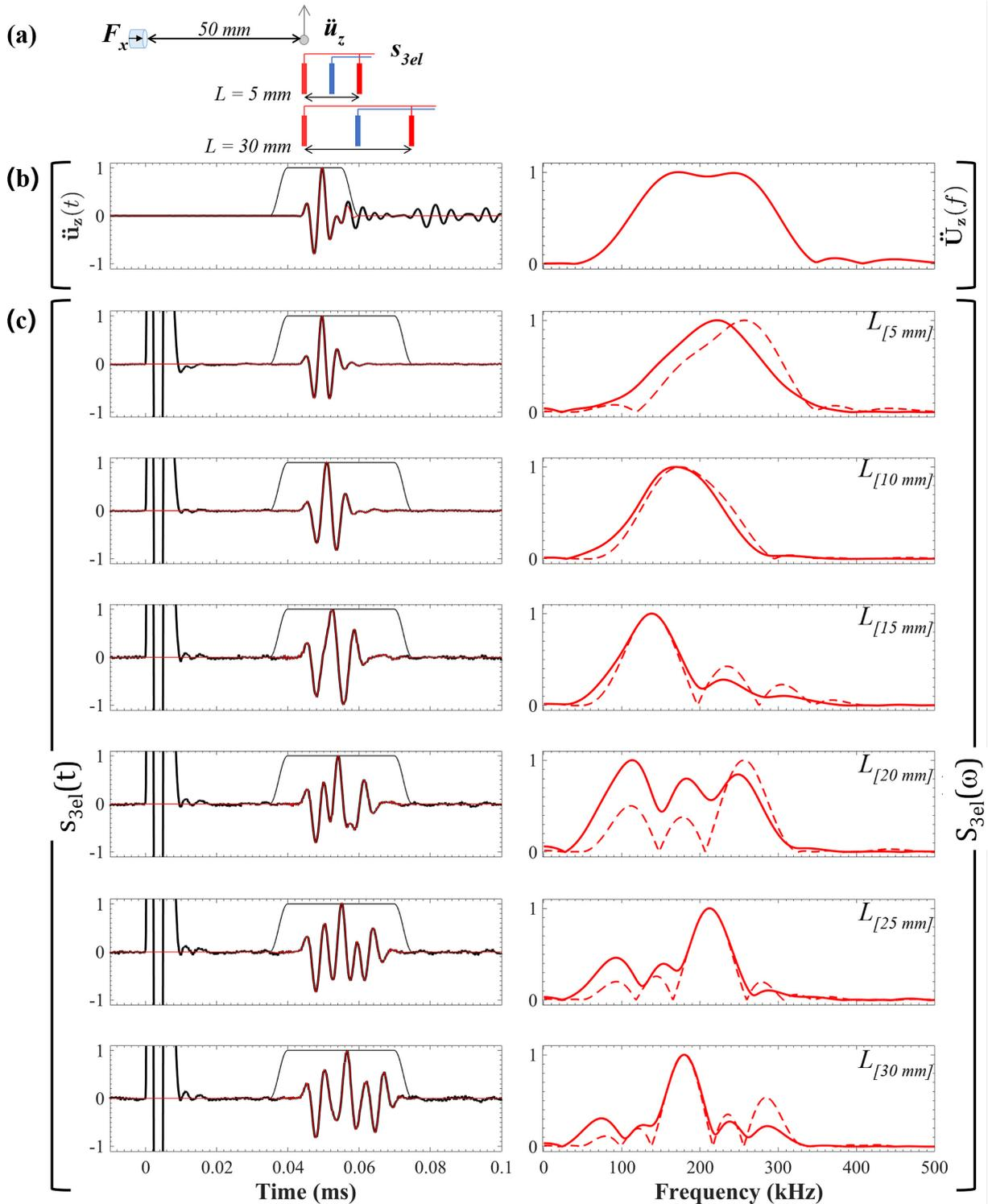
**Figure 7.** (a) Sketch of the acquisition for the three-electrode array. Outer and middle electrodes are displaced so that  $L$  varies from 5 to 30 mm. (b) Seismic acceleration acquired at an offset of 50 mm (top) followed by (c) seismoelectric recordings for the different offset (left) and corresponding normalized observed (plain lines) and predicted (dashed lines) spectra (right).
