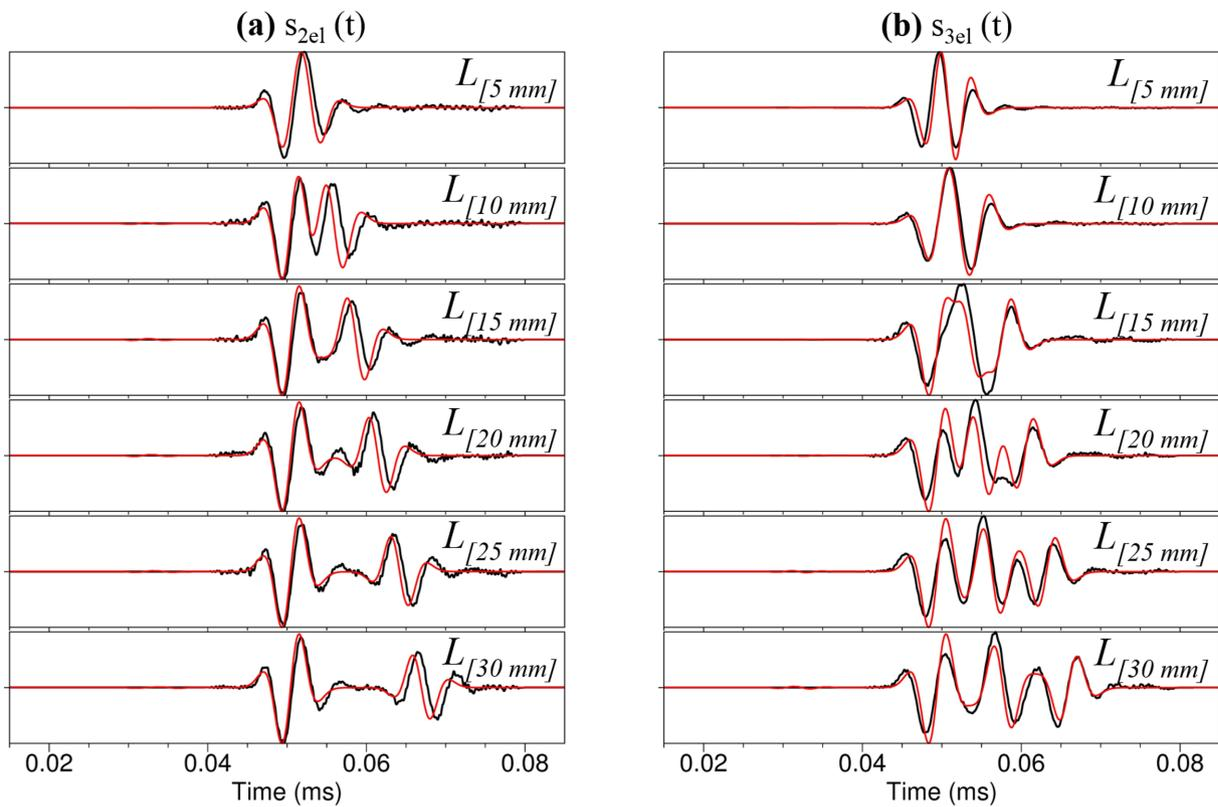
**Figure 13.** Numerical (red curve) and laboratory (black curve) normalized seismoelectric data acquired for an inner electrode located at 50 mm from the 200 kHz source. The two-electrode (a) and three-electrode (b) configurations are compared for various array lengths  $L$ . Numerical computations were made considering homogeneous material I.
