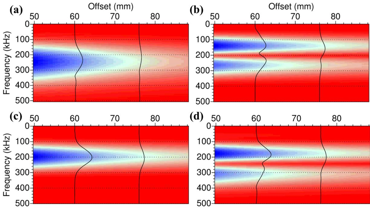
**Figure 12.** Spectral amplitudes versus offset of the acceleration (a) and seismoelectric synthetic data obtained using the two-electrode (b), three-electrode (c) and five-electrode (d) configurations. The black curves show the experimental spectra obtained for two traces located at 60 and 76 mm.
