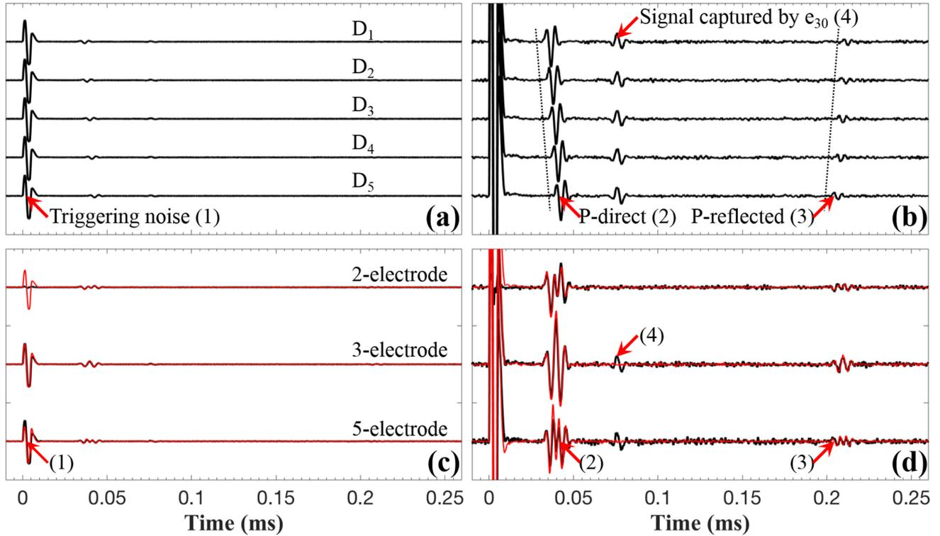
**Figure 2.** (a) Raw and (b) amplified voltage differences  $D_n(t)$  for five inner electrode locations (50–60 mm). Comparison of raw (c) and amplified (d) local electrical potential differences  $\tilde{s}_{iel}(t)$  measured at  $e_1$  as inner electrode and using a reference electrodes  $e_{30}$  (red lines) and  $s_{iel}(t)$  obtained directly from different connections (blue lines) for the 2- (top), 3- (middle) and five-electrode (bottom) arrangements with an array length  $L$  of 10 mm.
