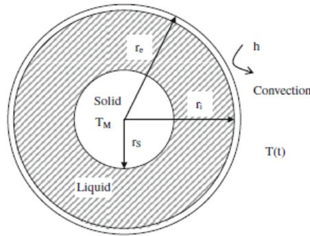
Fig. 2. Melting inside a spherical capsule. Adapted from [9].
