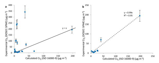
Figure 1: Calculated surface concentration for an air velocity of 0.20 m.s<sup>-1</sup> from the emission chamber results versus surface concentration measured by DOSEC®-SPME method (a) all 19 materials (b) raw materials.
