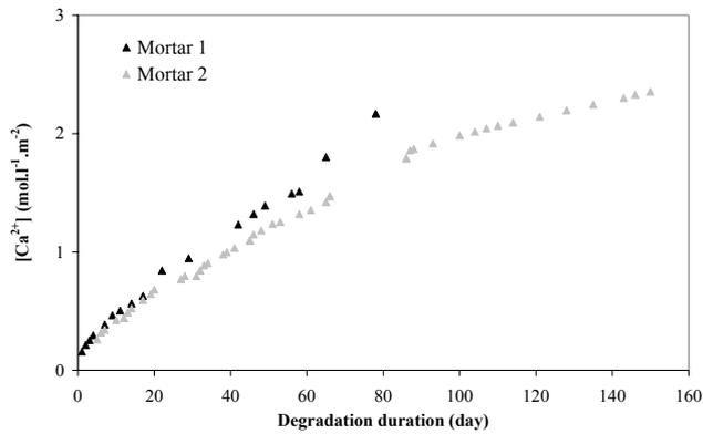
Fig. 6 - Calcium leached during attack of mortar 1 and 2.
