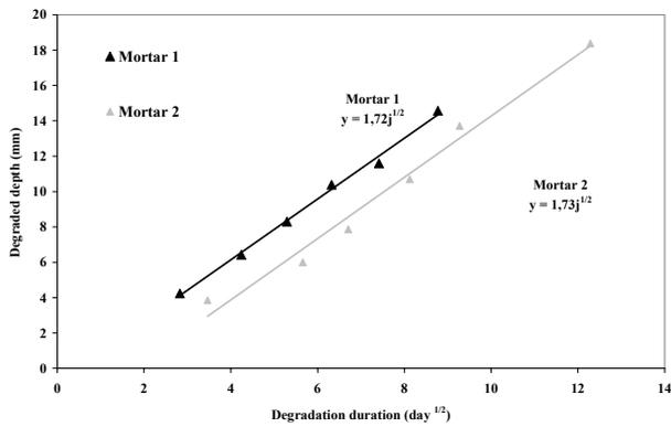
Fig. 5 - Degraded depth versus aggressive period.
