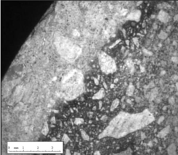
Fig. 3 - Videomicroscope image of mortar 1 degraded depth.
