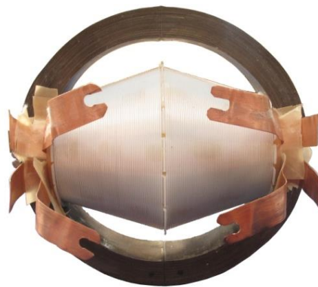
Figure 13: Picture of the completed resonant magnetic core pulsed transformer
