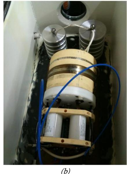
Figure 18: (a) Electrical scheme of the test and (b) photo of the real experimental arrangement without oil
