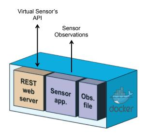
Fig. 4: High-level composition of a Virtual Sensor Container (VSC) packaged into a Docker container
