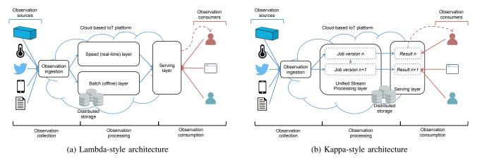
Fig. 3: High-level overview of two Cloud-based IoT platforms following the Lambda and Kappa architectures, respectively
