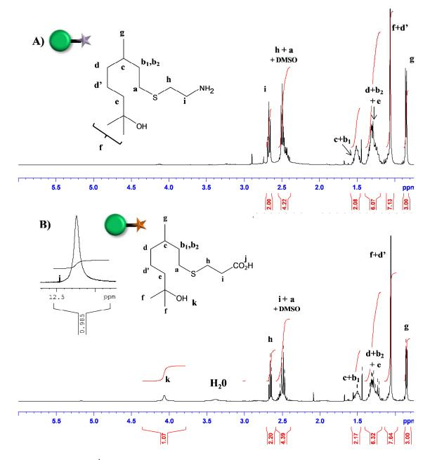
Figure 1. <sup>1</sup>H NMR spectra Terpene 1 (A) and Terpene 2 (B) (in DMSO-*d*6).
