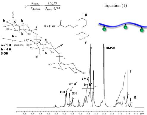
**Figure 5.** <sup>1</sup>H NMR spectrum of Dext-*graft*-DHM<sub>10.4</sub> in DMSO-*d*6.
