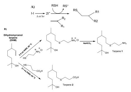
Scheme 2. (A) General principle of radical thiol-ene chemistry using an initiator (I-I) and a thiol transfer agent (RSH); (B) Derivatization of dihydromyrcenol (DHM) terpene by thiol-ene chemistry to produce functional Terpene 1 and Terpene 2.
